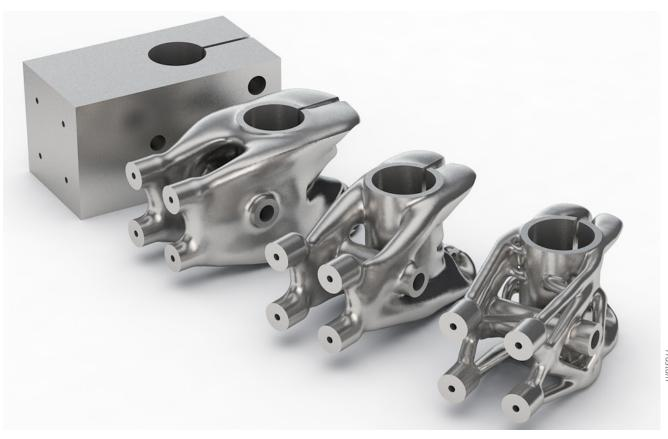
» Frustum's Generate was used to optimize this part for 3D printing. The designer was able to precisely control how this complex geometry was built, to take full advantage of the latest additive manufacturing capabilities.
