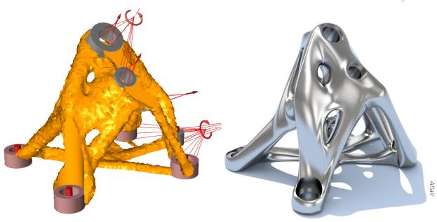
» This engine mount was designed using Altair solidThinking Inspire. Starting with a block of material, factoring in constraints, forces, and material type, the software creates optimized geometry for the part.
